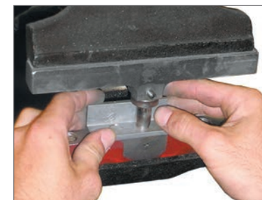
Bench vise used vertically as a press.
