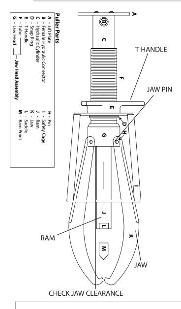
DUE TO VARIANCES IN JAW FORGINGS, IT IS ADVISABLE TO CHECK JAW CLEARANCE BETWEEN RAM AND JAW NEAR THE JAW PIN AREA WHEN CHANGING JAWS.
